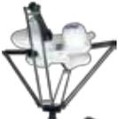
**Adept Quattro™** parallel (4-arm) robots are capable of up to 2,000 picks per hour. Fast, nimble, energy-saving and smooth, they minimize product breakage and maximize throughput.
