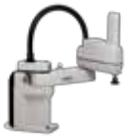
**Adept Cobra™** high-speed, high precision SCARA (4-axis) robots lead the category in assembly, kitting, packaging and other material-handling applications.
